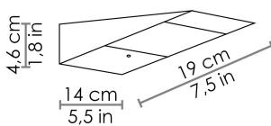
Wall lamps in dark grey painted die-cast aluminium, with a polycarbonate diffusor. The high IP rating (IP54) makes the lamps ideal for indoor and outdoor use. The lamps are fitted with a solar panel that auto-charges the battery, a dusk sensor and a motion sensor (this solar product requires no electrical connection). Replaceable battery.
